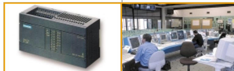
Alarm peaks are transferred to a PLC or a control room through 4-20 mA
